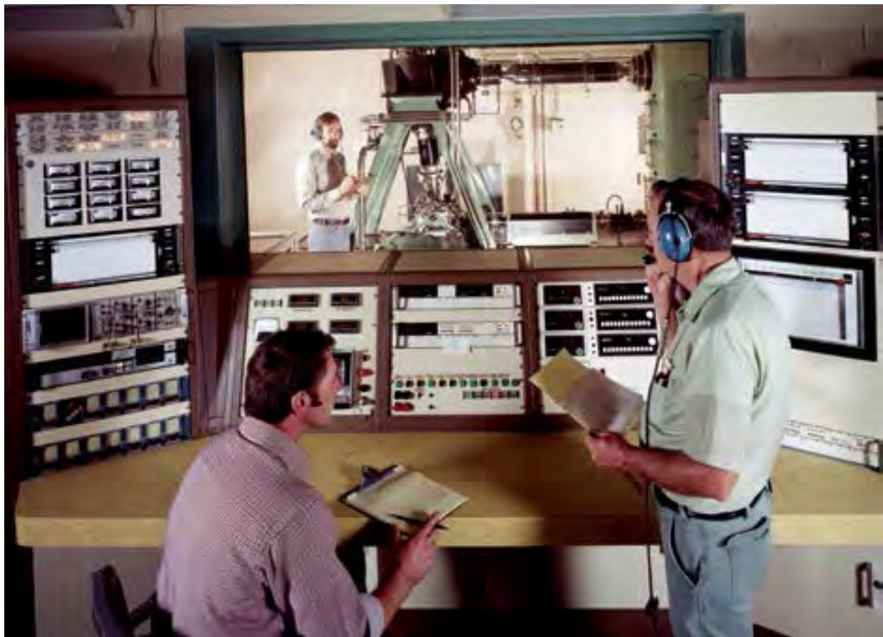
Image 302: Helicopter Transmission Rig in the Engine Research Building (GRC-1978-C-4355).
