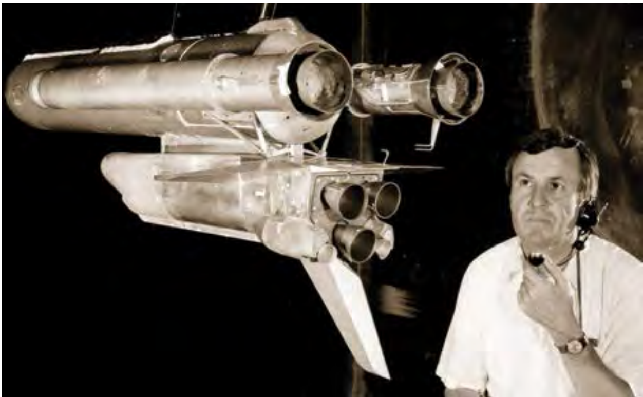
Image 280: Ken Baskin checks a complete 2.25-scale model of the shuttle in the 10×10 test section during July 1975 (GRC-1975-C-02011).
