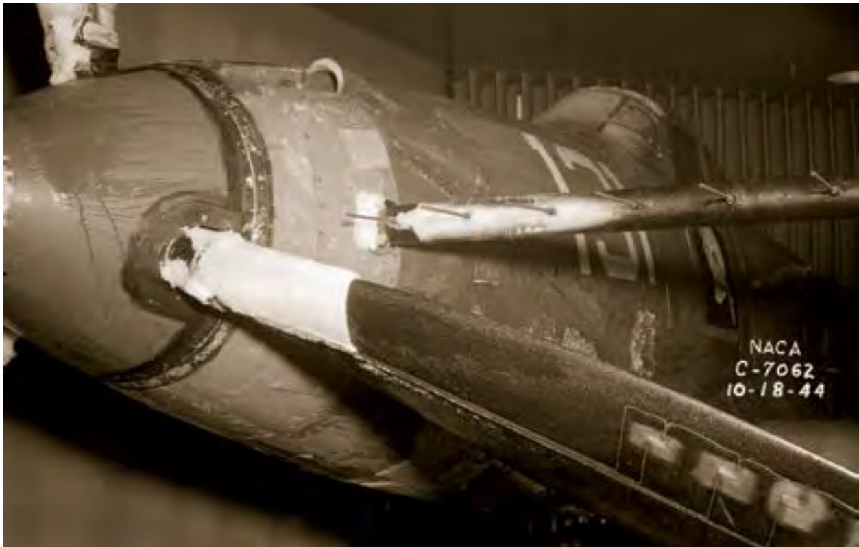
Image 50: P-39 Airacobra fuselage being tested in the IRT in October 1944 (GRC-1944-C-7062).
