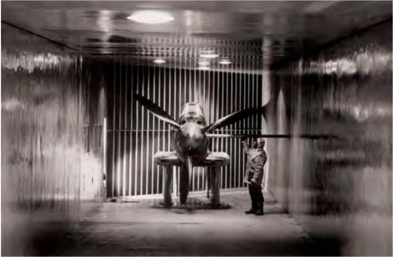
Image 68: P-38 Lightning fuselage in the IRT during March 1945 (GRC-1945-C-8832).
