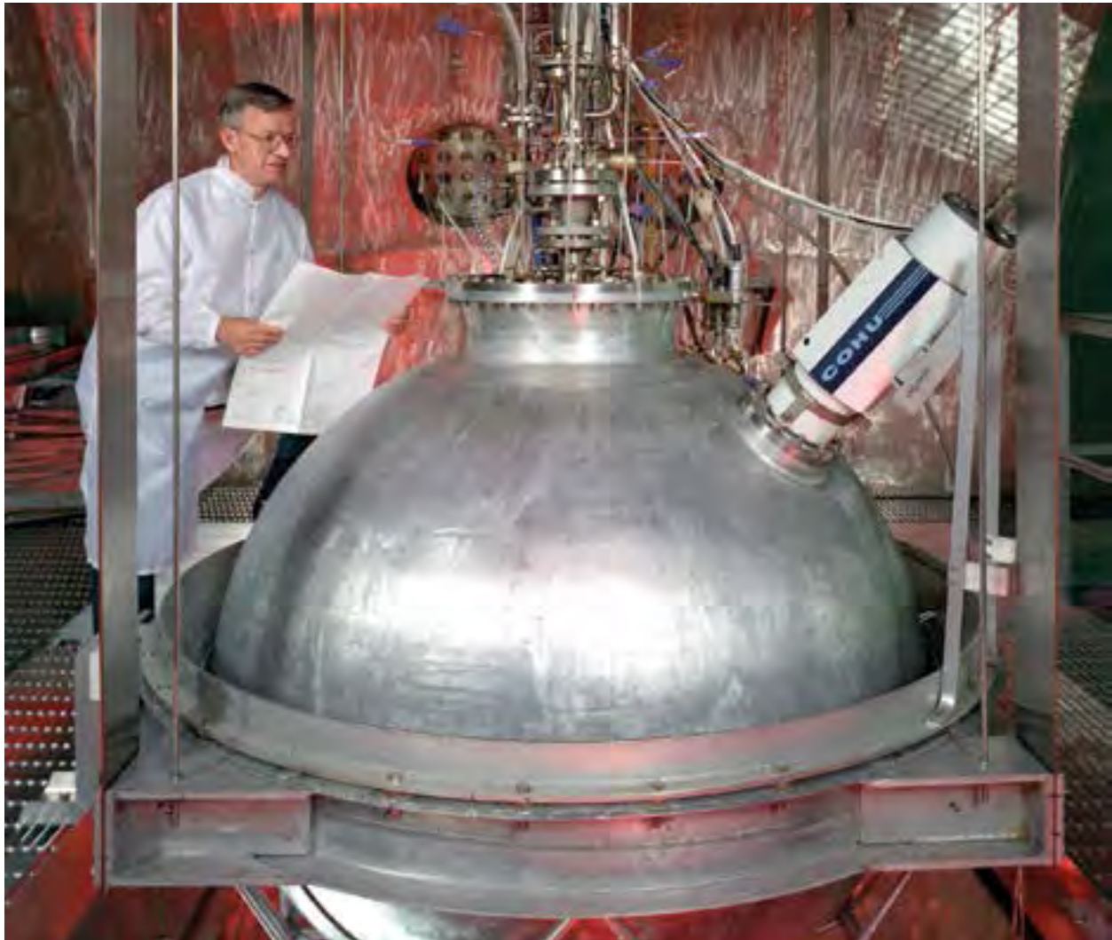
Image 319: William Klein examines settings for the slush hydrogen test rig in the K Site vacuum chamber during June 1991 (GRC-1991-C-07458).
