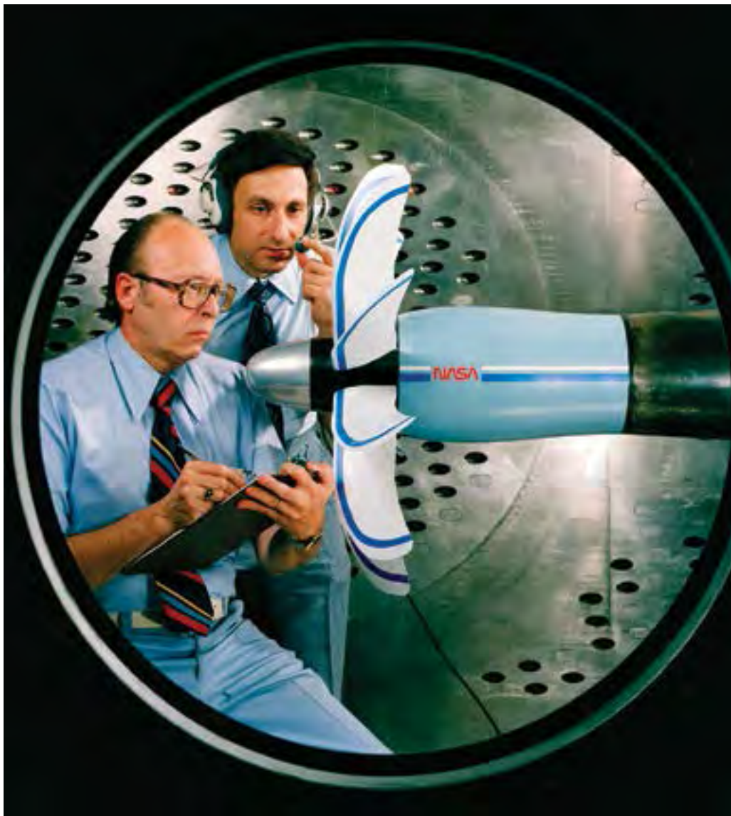
Image 273: Glenn Mitchell (left) and Oral Mehmed with a Hamilton Standard SR–6 propfan in the 8×6 test section (GRC–1980–C–04620).
