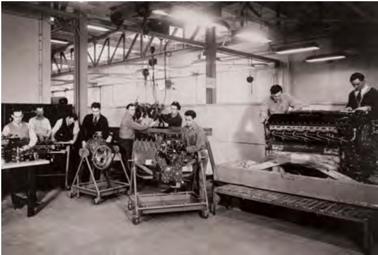
Image 63: A representative from the Allison Engine Company instructs AERL mechanics on the operation of a basic Allison powerplant. The staff was taught how to completely disassemble and reassemble the engine components and systems (GRC-1943-C-03045).
