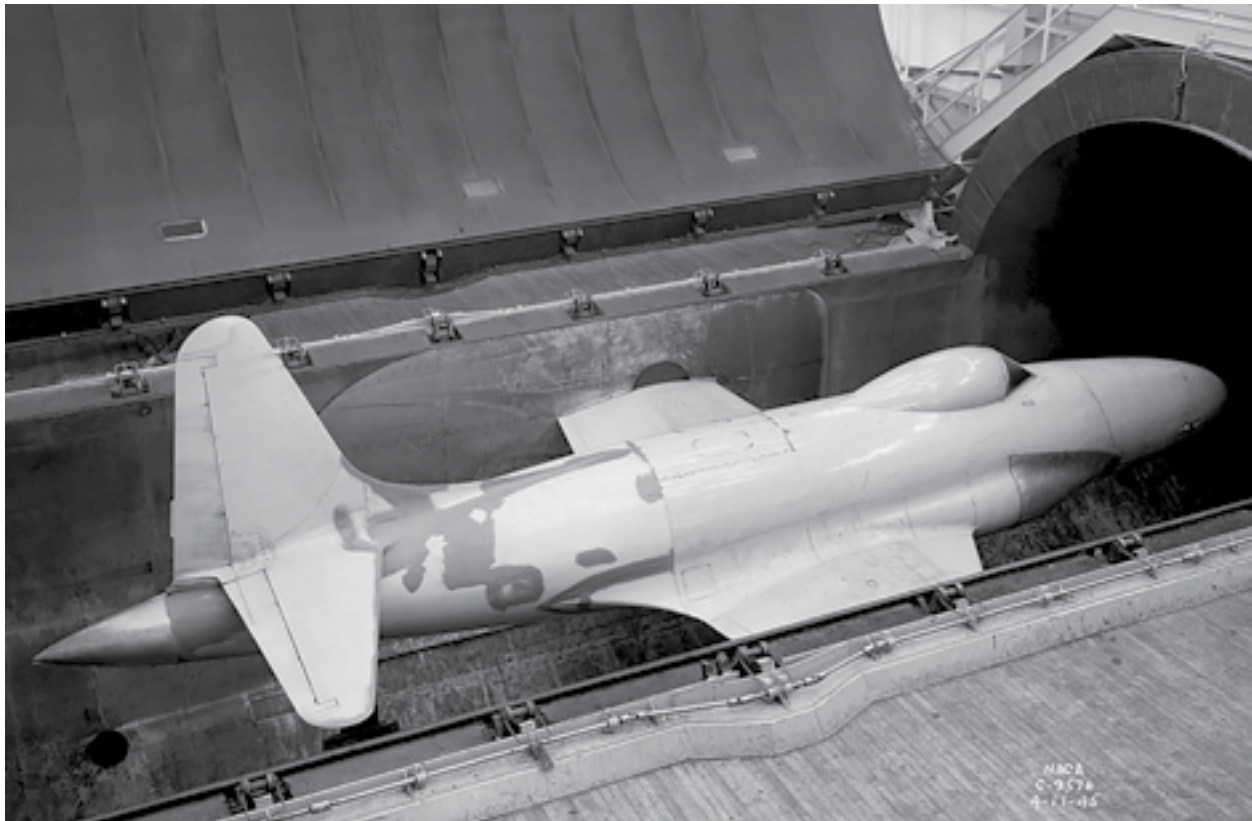
Image 74: Lockheed's YP-80A, powered by two General Electric I-40 turbojets, in the AWT test section in March 1945. The P-80 was the first U.S. aircraft to fly faster than 500 mph (GRC-1945-C-09576).
