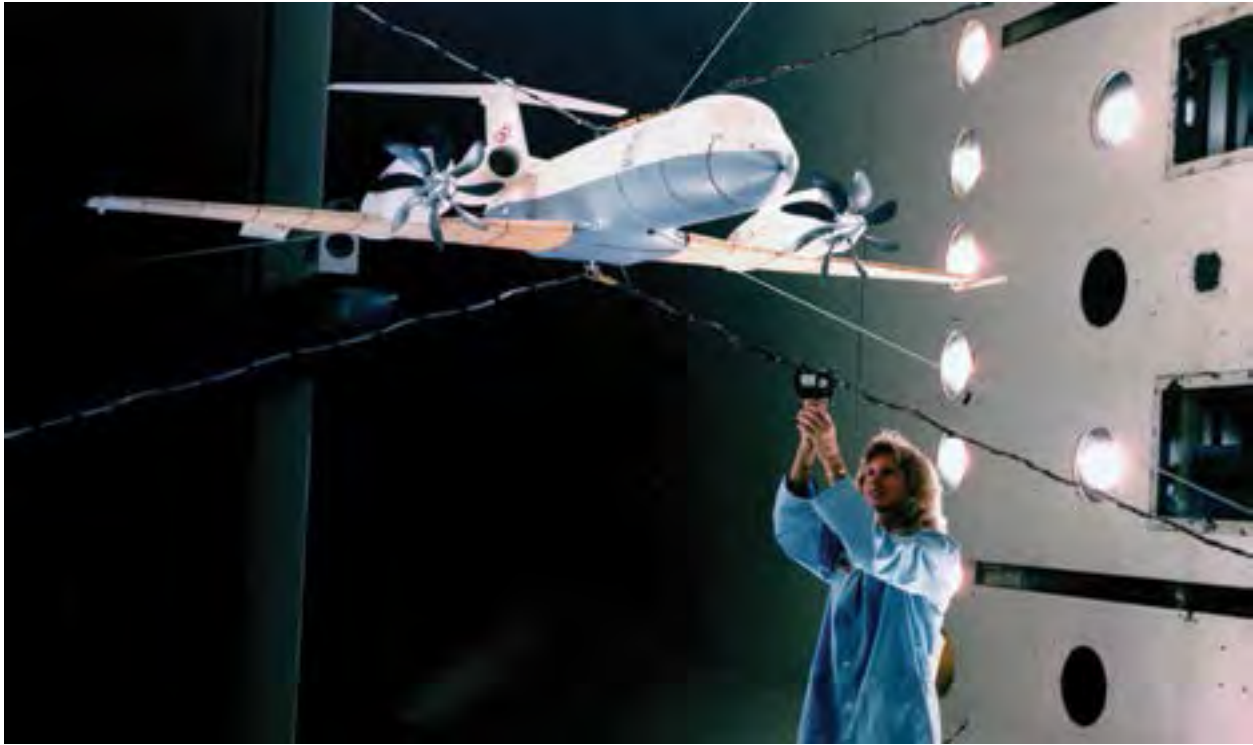
Image 297: A Propfan Test Assessment model is tested for flutter in a Langley wind tunnel during October 1985 (GRC-1985-C-07896).
