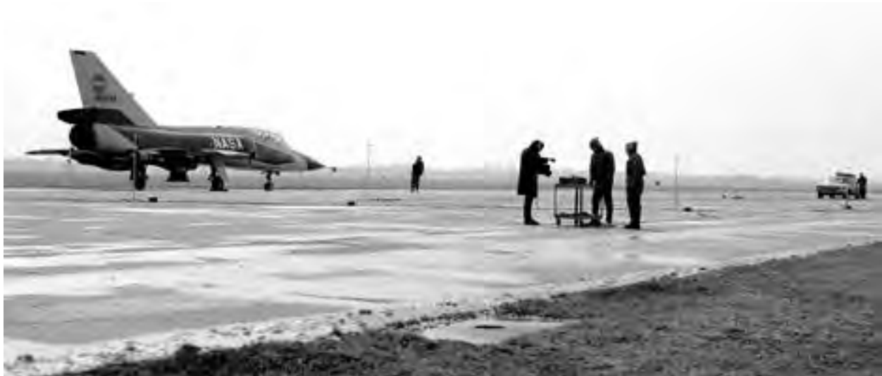
Image 218: Lewis researchers take ground-based noise measurements from the F-106B (GRC-1971-C-00775).
