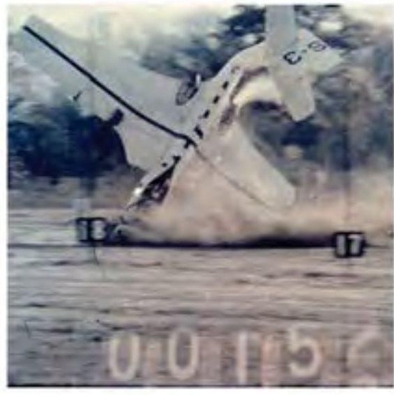
Image 140: A 1955 example of Bill Wynne's innovative visual timekeeping method for the Crash Fire Program (GRC-C-1955-38196).
