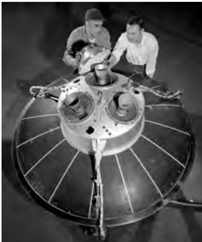
Image 174: Gale Butler examines the Mercury capsule's retrograde rockets prior to a test run inside the AWT (GRC-1960-C-53146).
