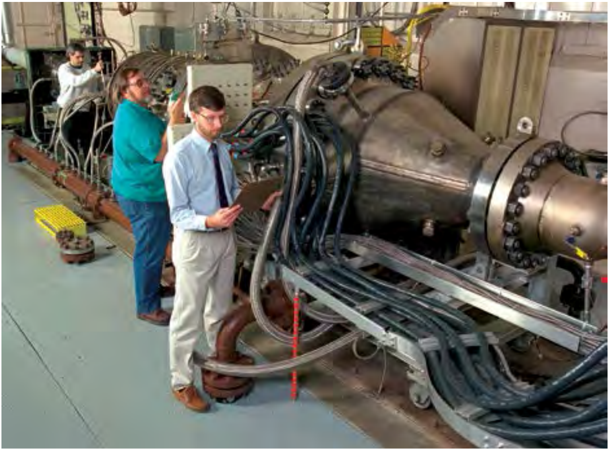
Image 341: Advanced Subsonic Combustion Rig in the Engine Research Building (GRC-1999-C-00249).
