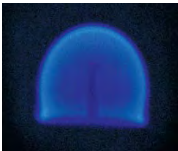
Image 350: A candle flame in a microgravity environment (GRC-1998-C-00486).
