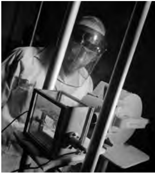
Image 200: Bob Siegel with a test rig for high-speed filming of liquid behavior in microgravity in the 8x6 wind tunnel (GRC-1960-C-54149).
