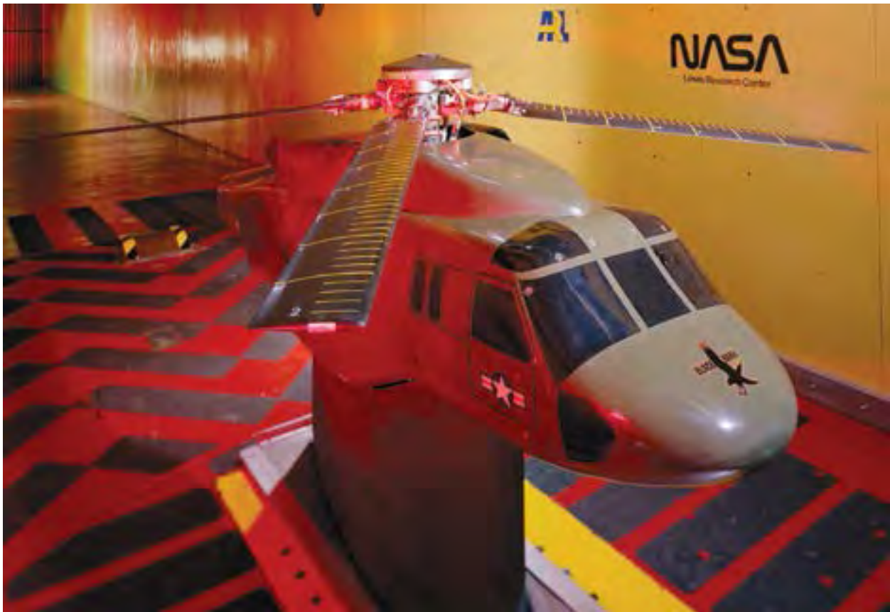
Image 299: Rotorcraft model installed in the IRT (GRC-1993-C-03670).
