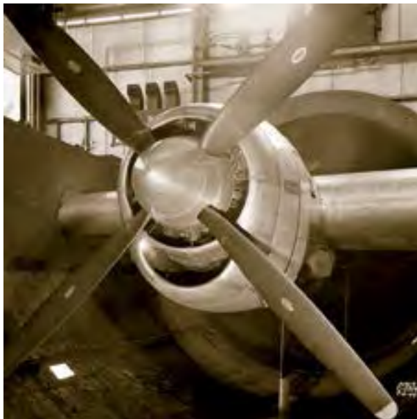
Image 65: Wright R-3350 installed in the AWT test section on 4 July 1944 (GRC-1944-C-05554).
