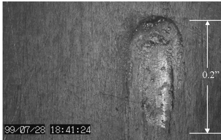
Figure 13 -- Main Combustion Chamber Ding
