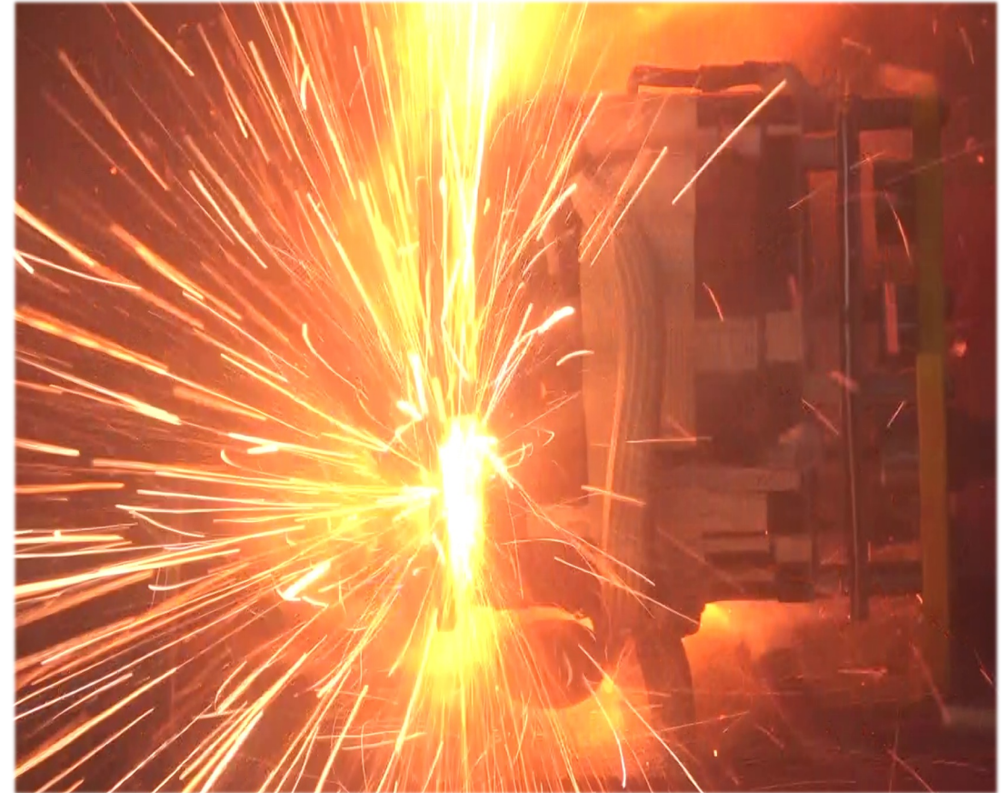
Figure: video frame capture moments after initiating thermal runaway of Cell 8 via axial nail penetration.
