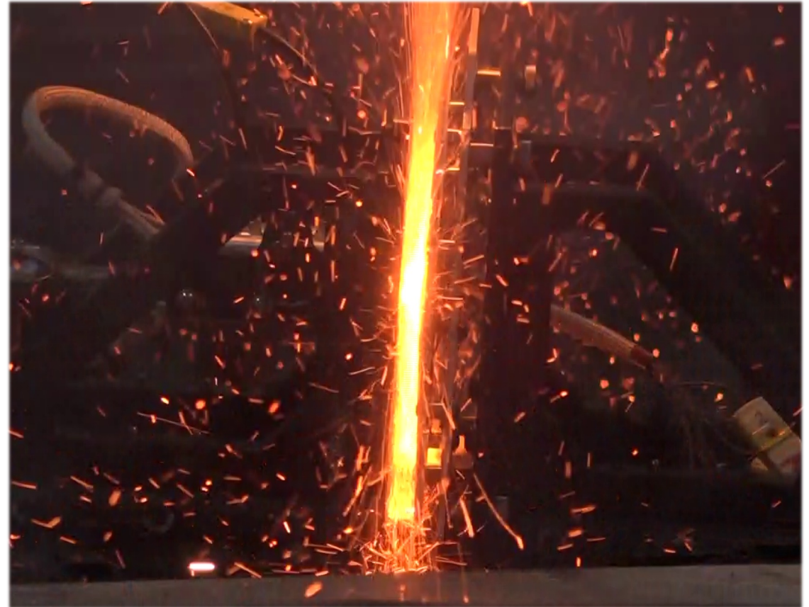
Figure: video frame capture moments after initiation of thermal runaway via axial nail penetration.
