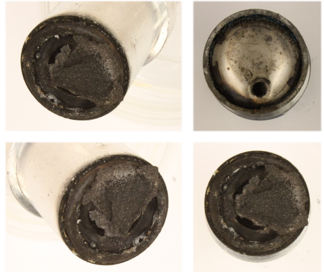
Figures: various views of “spent” Samsung 50S cell following blast plate test at pre-set distance.
