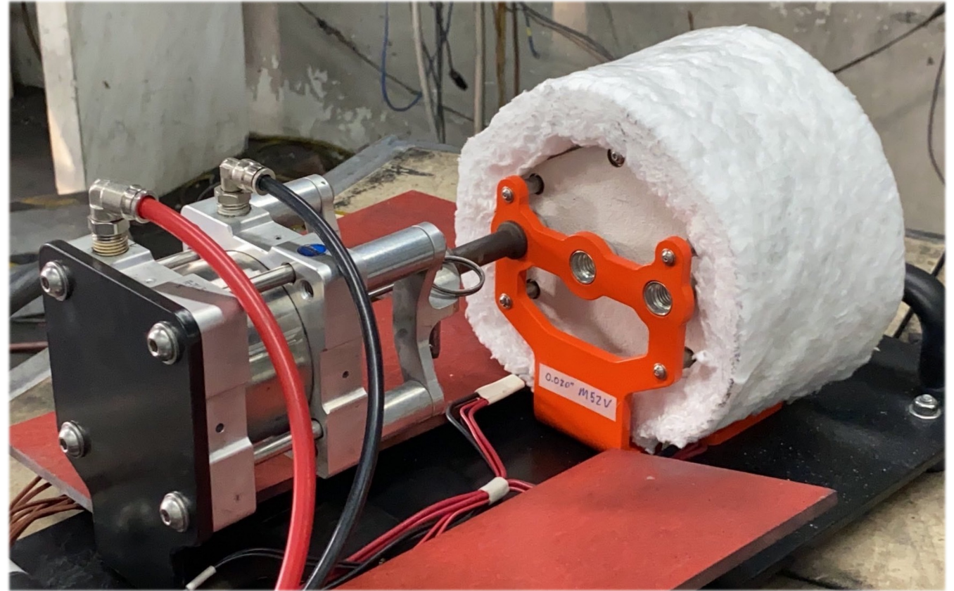
Figure: For elevated temperature runs, batteries were insulated and thermally conditioned. Insulation was removed immediately prior to TR.
