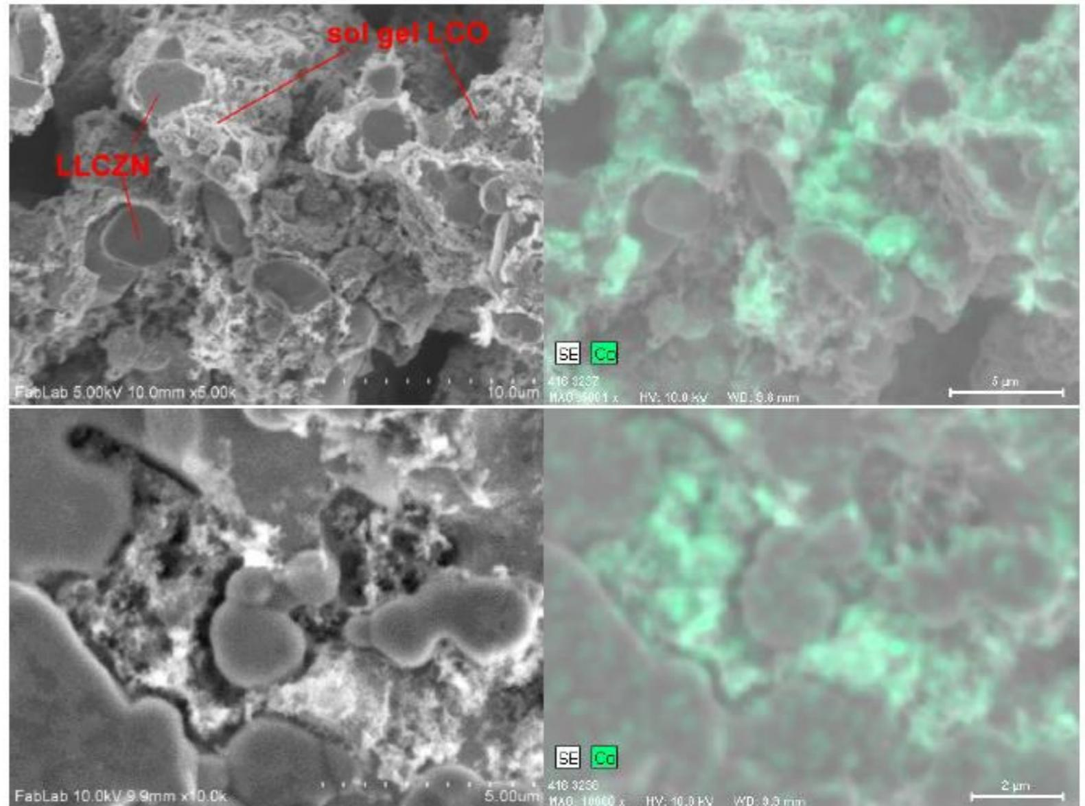
Infiltrated LCO as well as a number of cathode materials into the porous garnet structure
