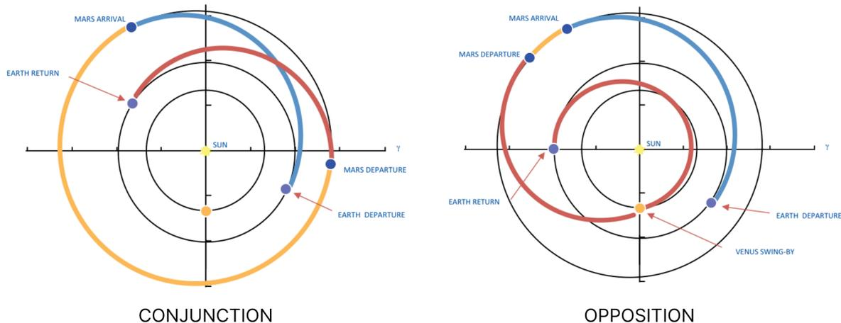
**Figure 2-8. Illustration of Conjunction- and Opposition-Class Mars Trajectories**
