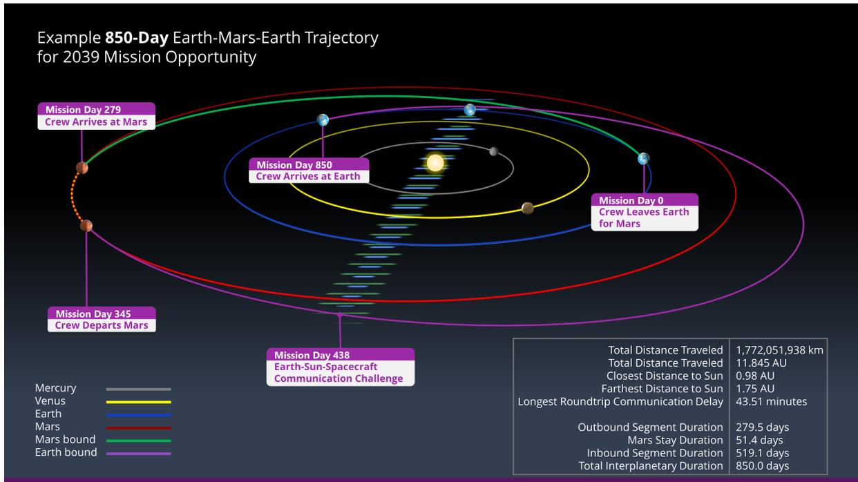
**Figure 2-7. Roundtrip Mars Mission Distance in Perspective (AU, Astronomical Unit)**
