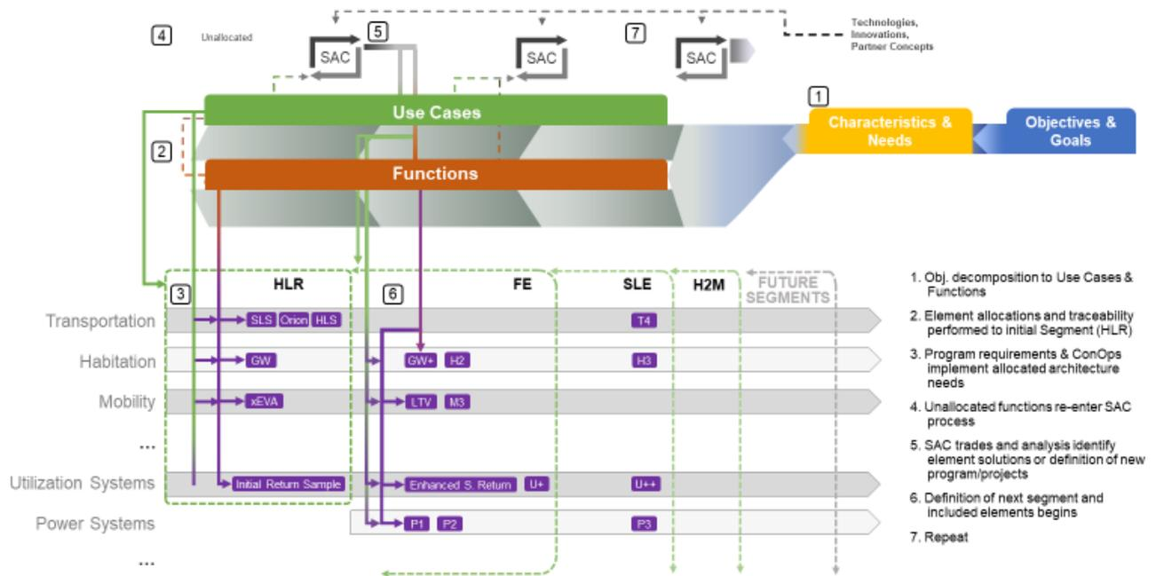
Figure 1-7. Illustration of the Architecture Definition Process
