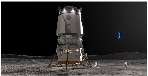
Figure 3-18. Human Landing System—One of the Integrated Lander Configurations as Awarded (Image credit: Blue Origin)
