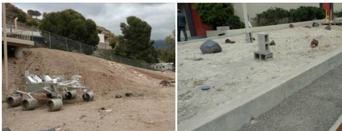
The Mars Yard (left) and Robotics Arena (right) are the primary designated outdoor testing areas within the NASA JPL facility. These areas are used to test rovers as well as other robotic devices in appropriate outdoor settings that mimic the natural environment, but also in close proximity to fabrication and development facilities.
