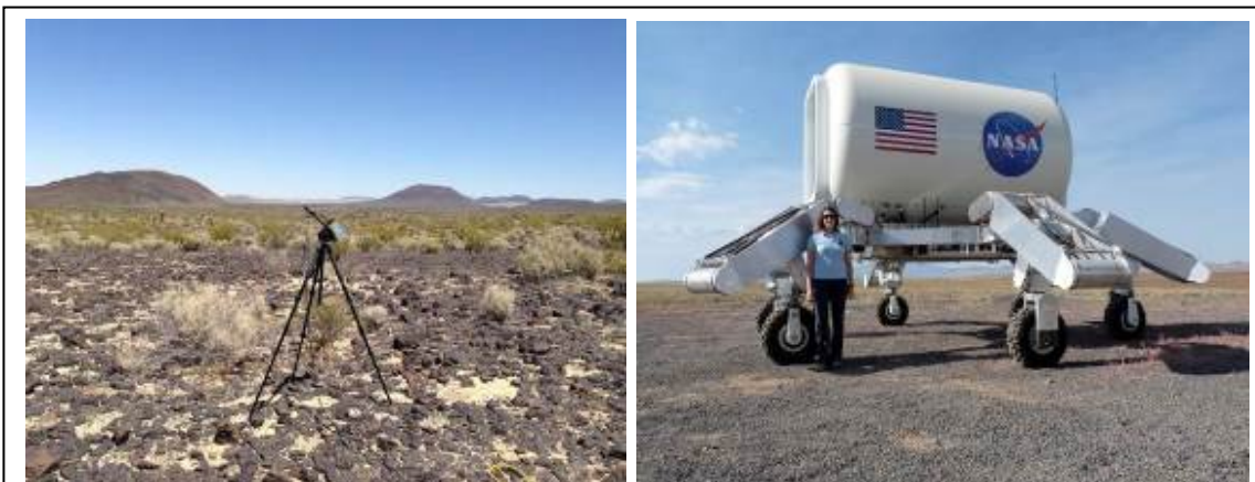
Small-scale testing activities in the Arroyo Seco have ranged from camera imaging (left; representative photograph from the Mojave Desert) to ATHLETE Rover testing (right; representative photograph). These activities are currently carried out in the Arroyo Seco under individual agreements with the City of Pasadena and other relevant state and/or Federal agencies (e.g., Federal Aviation Administration [FAA] for quadrotor flights).
