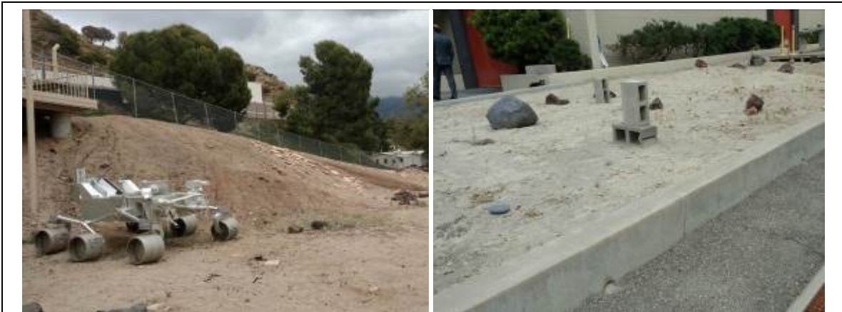
The Mars Yard (left) and Robotics Arena (right) are the primary designated outdoor testing areas within the NASA JPL facility. These areas are used to test rovers as well as other robotic devices in appropriate outdoor settings that mimic the natural environment, but also in close proximity to fabrication and development facilities.
