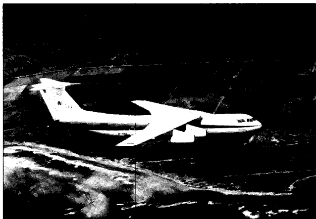
The Kuiper Airborne Observatory, a Lockheed C-141 aircraft modified to carry a 36-inch diameter telescope, flies above most of Earth's atmosphere at 41-45,000 feet to perform astronomical observations of the planets and stars at the infrared wavelength.
