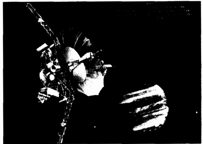
Artist's concept of Galileo spacecraft to Jupiter which will use General Purpose Heat Source Radioisotope Thermoelectric Generators.
