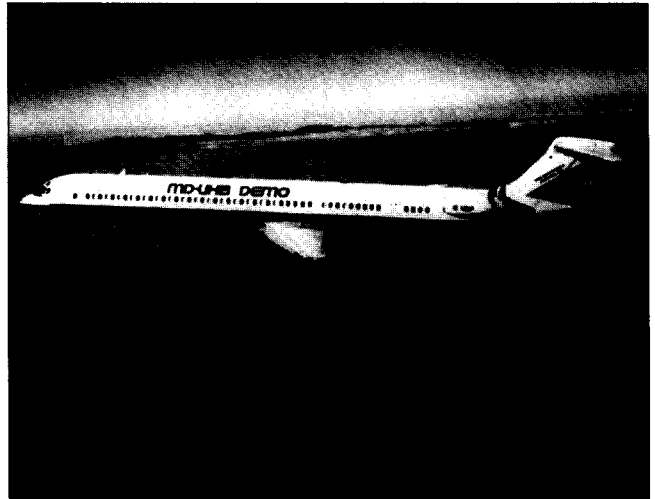
MD-80 aircraft flight testing the NASA/General Electric Unducted Fan (UDF) engine.
