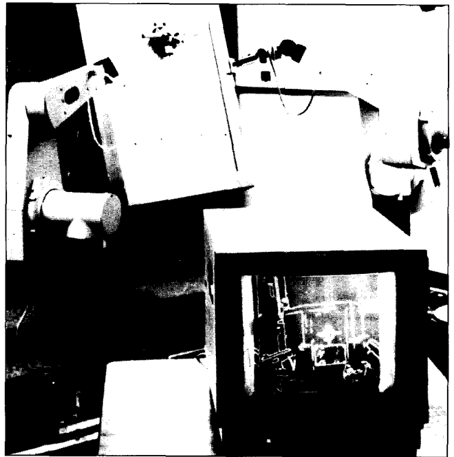
Automatic grappling of a spinning and tumbling satellite using robot vision and robot force-torque sensing.
