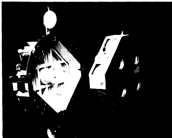
Attachment points of the Orbital Maneuvering Vehicle that will perform payload delivery to and retrieval from the Space Shuttle.
