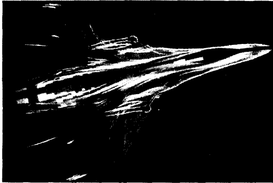
Computational Fluid Dynamics (CFD) flow field solution for the F-16 aircraft, generated by the Numerical Aerodynamic Simulation (NAS) system at Ames Research Center.
