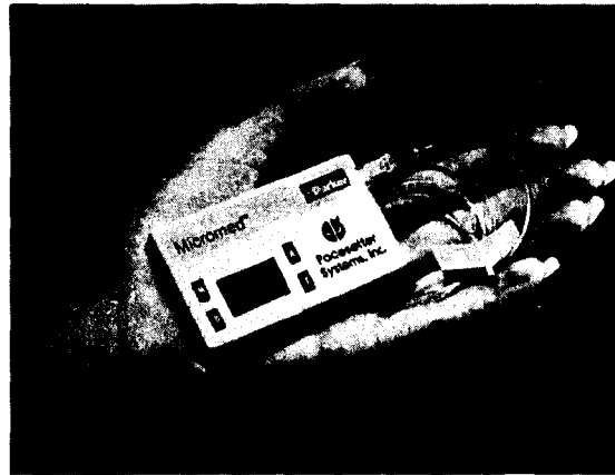
Based on technology developed for space systems, the Programmable Implantable Medication System will be used to deliver precise doses of medication to control diabetes and other diseases.
