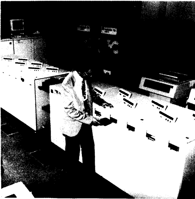
At the FAA Technical Center, a magnetic tape is fed into the new Host Computer System—an important element of the continuing modernization of air traffic control.
