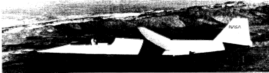
The remotely piloted HiMAT (Highly Maneuverable Aircraft Technology) (left) is providing NASA and the Air Force with supersonic flight data at twice the turn capability of present fighter aircraft. The oblique wing (below) can pivot from zero to 60 degrees in flight; it may provide future high-speed transport aircraft stable, economical flight characteristics at all speeds.
