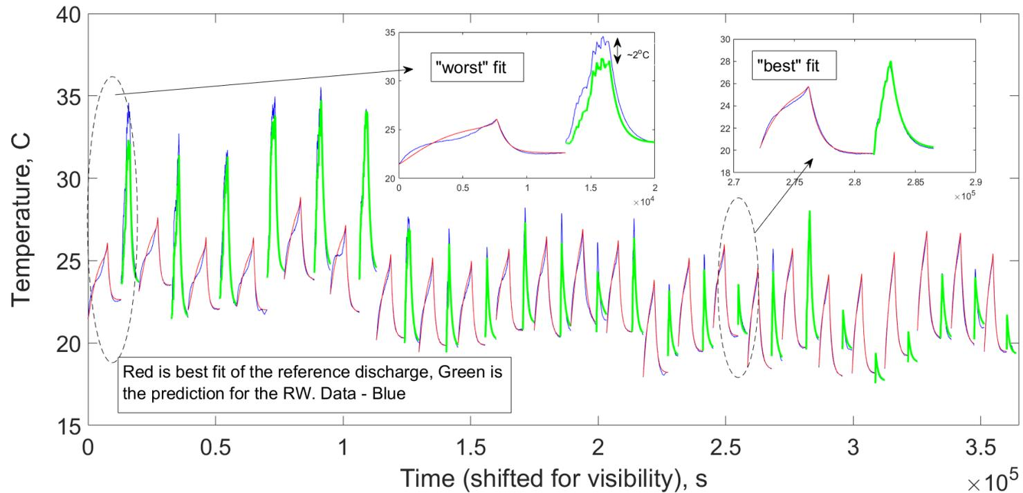
Fitting the TM to galvanostatic discharge data gives a decent prediction for RW data.
