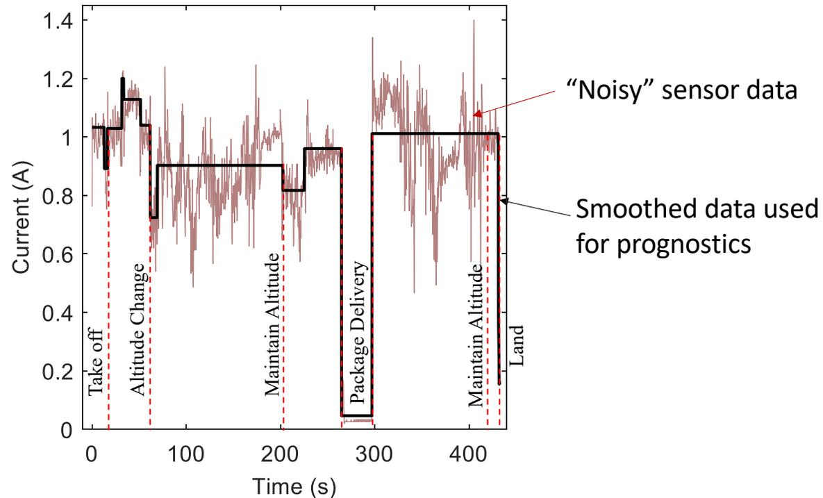
**Data pre-processing is needed for accurate estimation**
