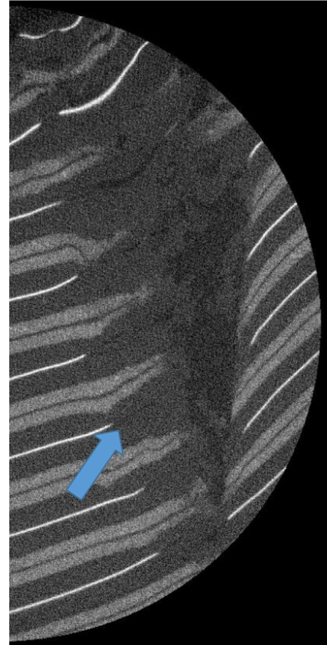
X-ray CT reveal Al and Cu PCCs withdrawn from the nail, thus reducing further short-circuiting. OCV measurement showed 4.07 V; cells retained voltage for over 10 months.
