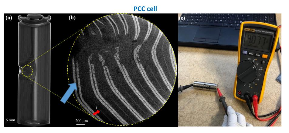
X-ray CT reveal Al and Cu PCCs withdrawn from the nail, thus reducing further short-circuiting. OCV measurement showed 4.07 V; cells retained voltage for over 10 months.
