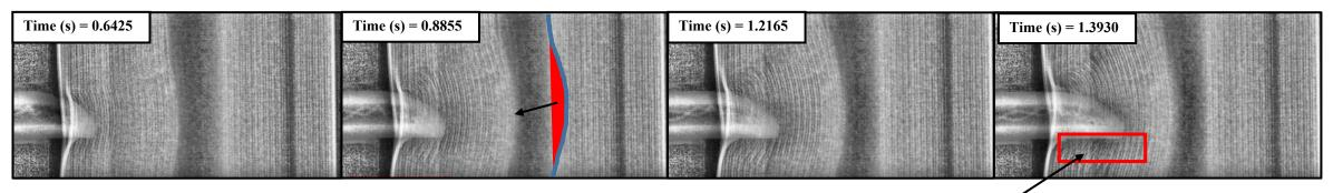
Electrode layers adjacent to nail splitting
