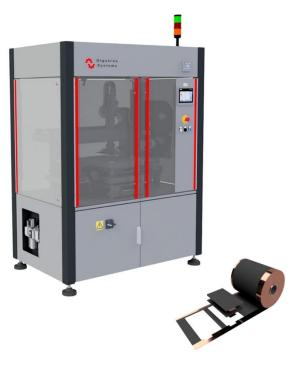
Digatron Systems ECU, electrode cutting unit, is an automatic electrode die cutting machine designed to punch electrodes from coated aluminium and copper rolls.
