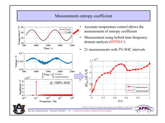
Measurement results from the multifunctional calorimeters
