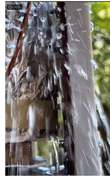
(c) t = 2682 s (just after the start of coolant release), T \sim 49 - 99^\circ\text{C}
