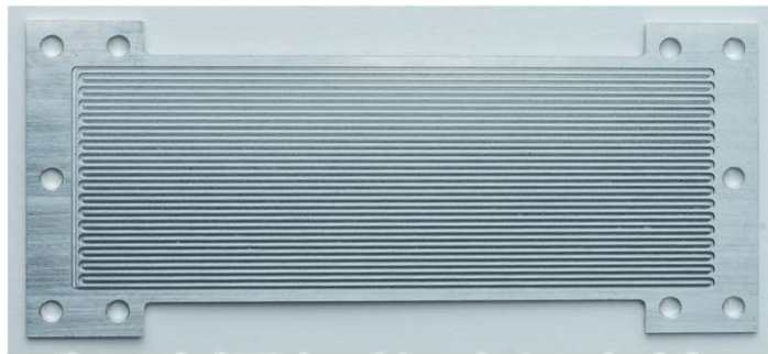
Photograph of OHP channels in an aluminum plate before brazing. Optimal performance requires custom channel routing for each heat map
