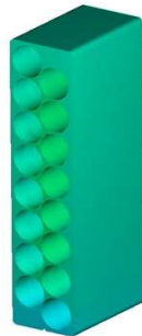
Aluminum OHP Model 16 W/K (<2K cell-cell)
