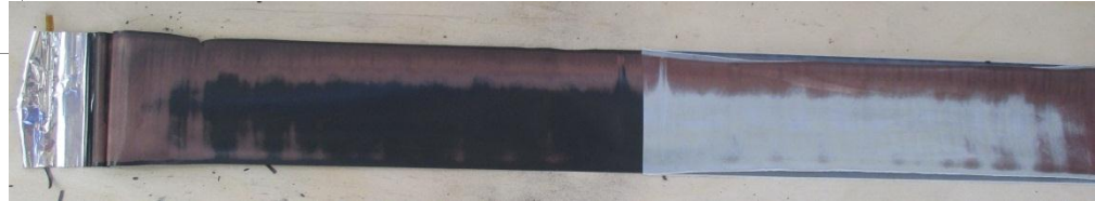
Positive electrode and separator showing copper deposit
