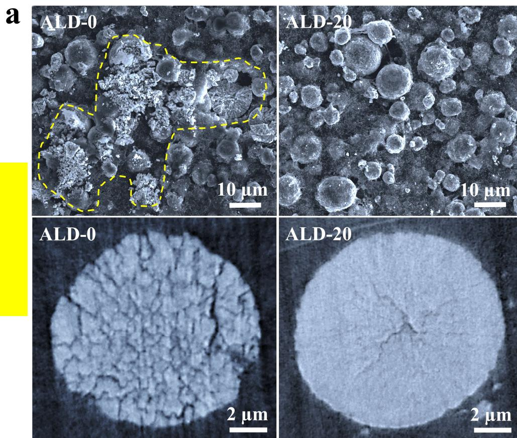
ALD  $\text{Li}_2\text{S}$  coating well protected NMC811 from cracking
