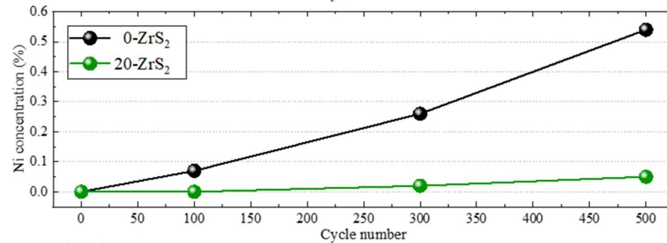
EDS revealed that the  $\text{ZrS}_2$  coating considerably reduce transition metal dissolution.
