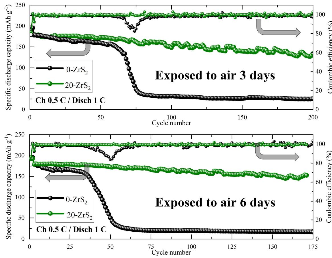
$\text{ZrS}_2$  coating is air-stable and can protect the NMC cathodes from degradation.
