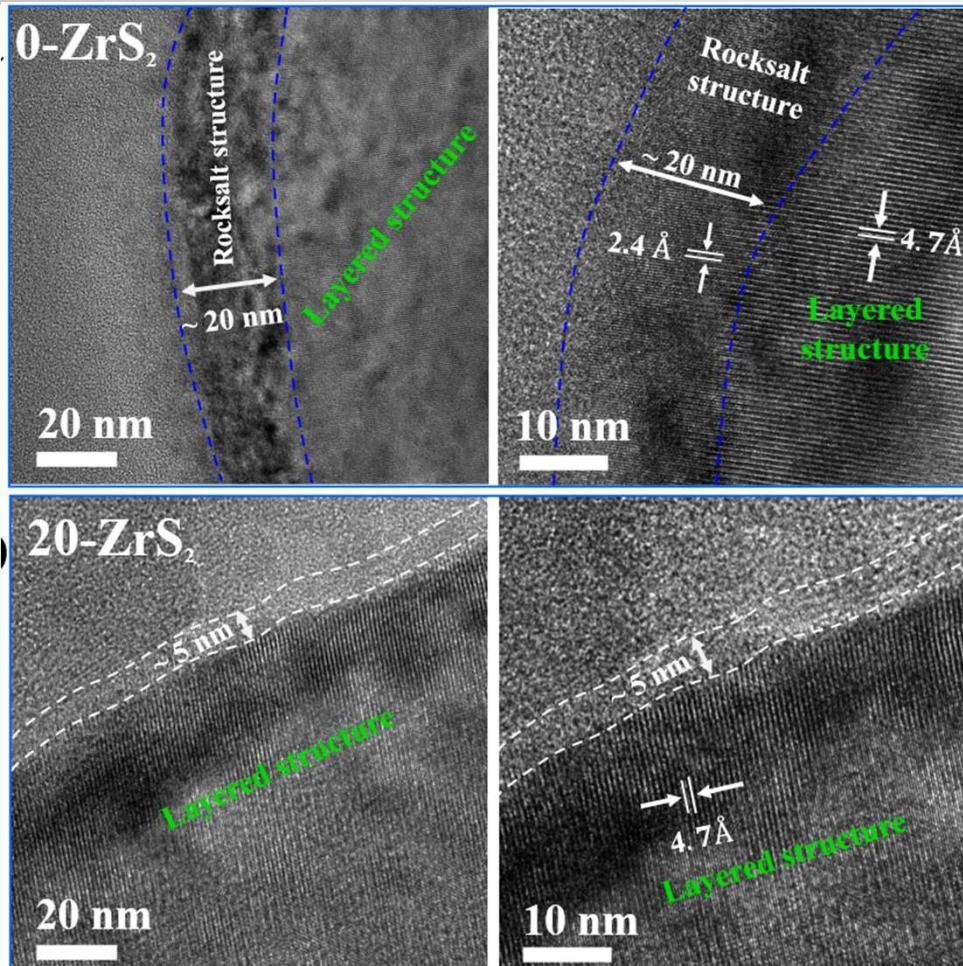
Evidently irreversible phase transition from layered structure to rocksalt structure.
