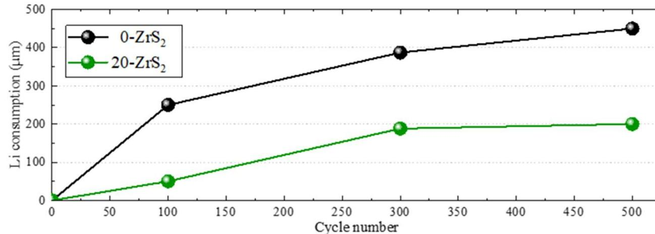
SEM observations disclosed that the  $\text{ZrS}_2$  coating remarkably helped mitigate the consumption of Li metal anodes.
