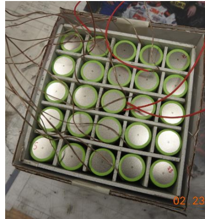
Bottom of the configuration with inserts between cells
