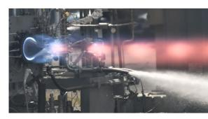
of propulsion development engineers at NASA developed and tested NASA's first full-scale rotating detonation rocket engine, or RDRE, an advanced rocket engine design that could significantly change how future propulsion systems are built. The RDRE differs from a traditional rocket engine by generating thrust using a supersonic combustion phenomenon known as a detonation. Engineers at Marshall confirmed data from RDRE hot fire tests conducted at Marshall's East Test Area.
