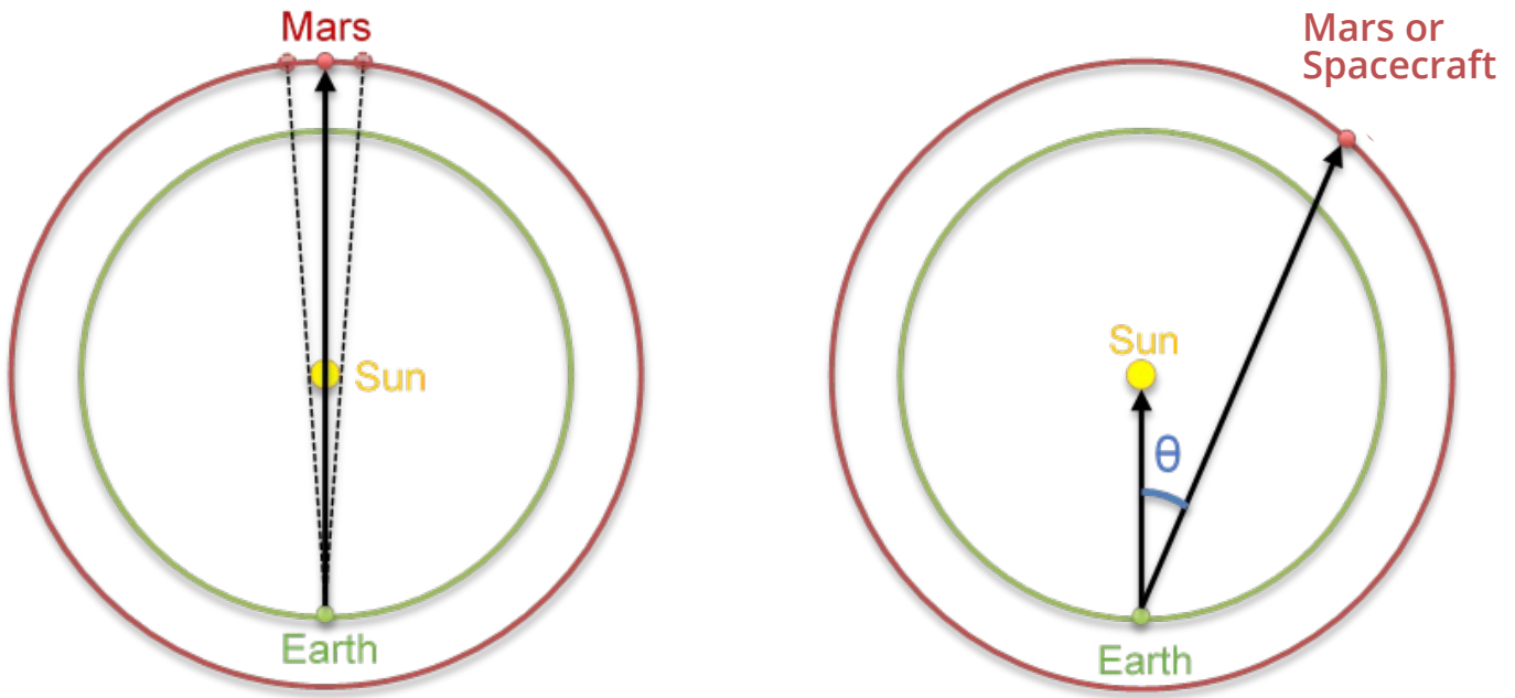
Figure 1. This diagram illustrates Earth-Sun-Mars conjunctions creating line-of-sight disruption between Earth and Mars (left) and the angle definition for communications disruption analysis (right).
