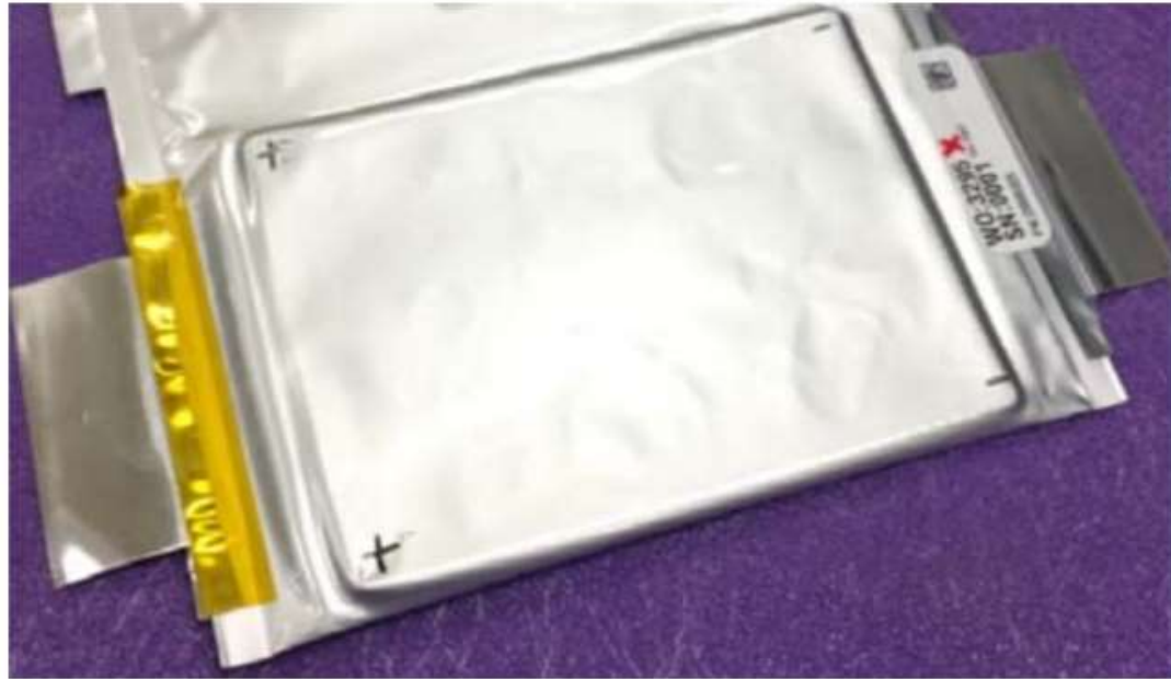
Figure 2 Soft prototype LTO cell with 0V storage capability
