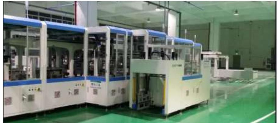
Li-Ion Battery pack assembly line in China
