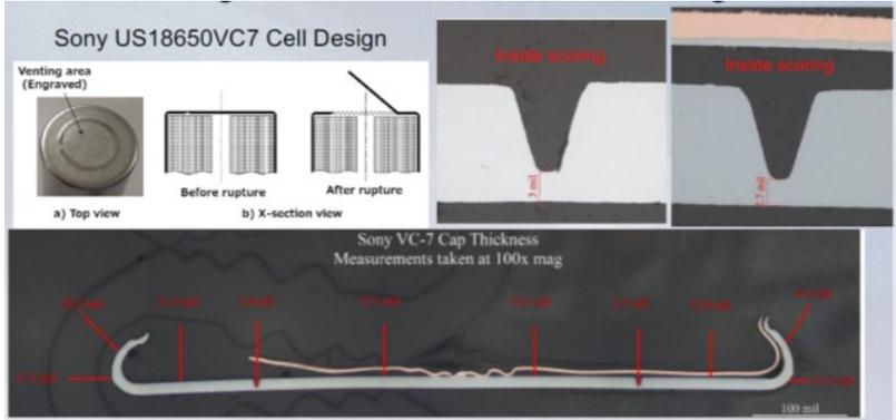
\*Side wall rupture during Cell Thermal runaway
