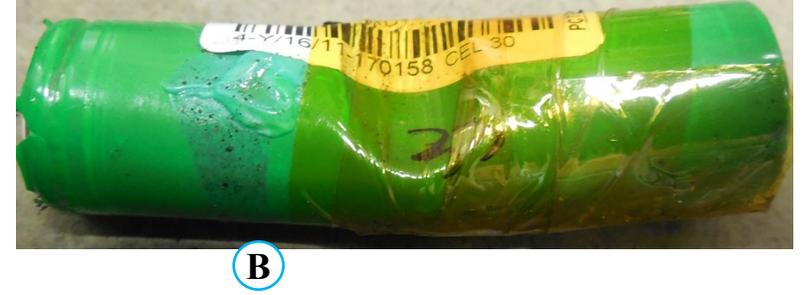
Cell structures were demolished by applied pressure.
