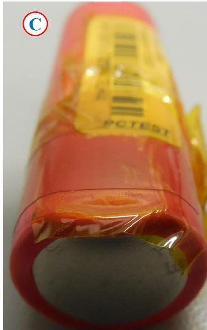
Cell structures were deformed by applied force, but that couldn't lead the cell to the ISC to generate heat and gas.
