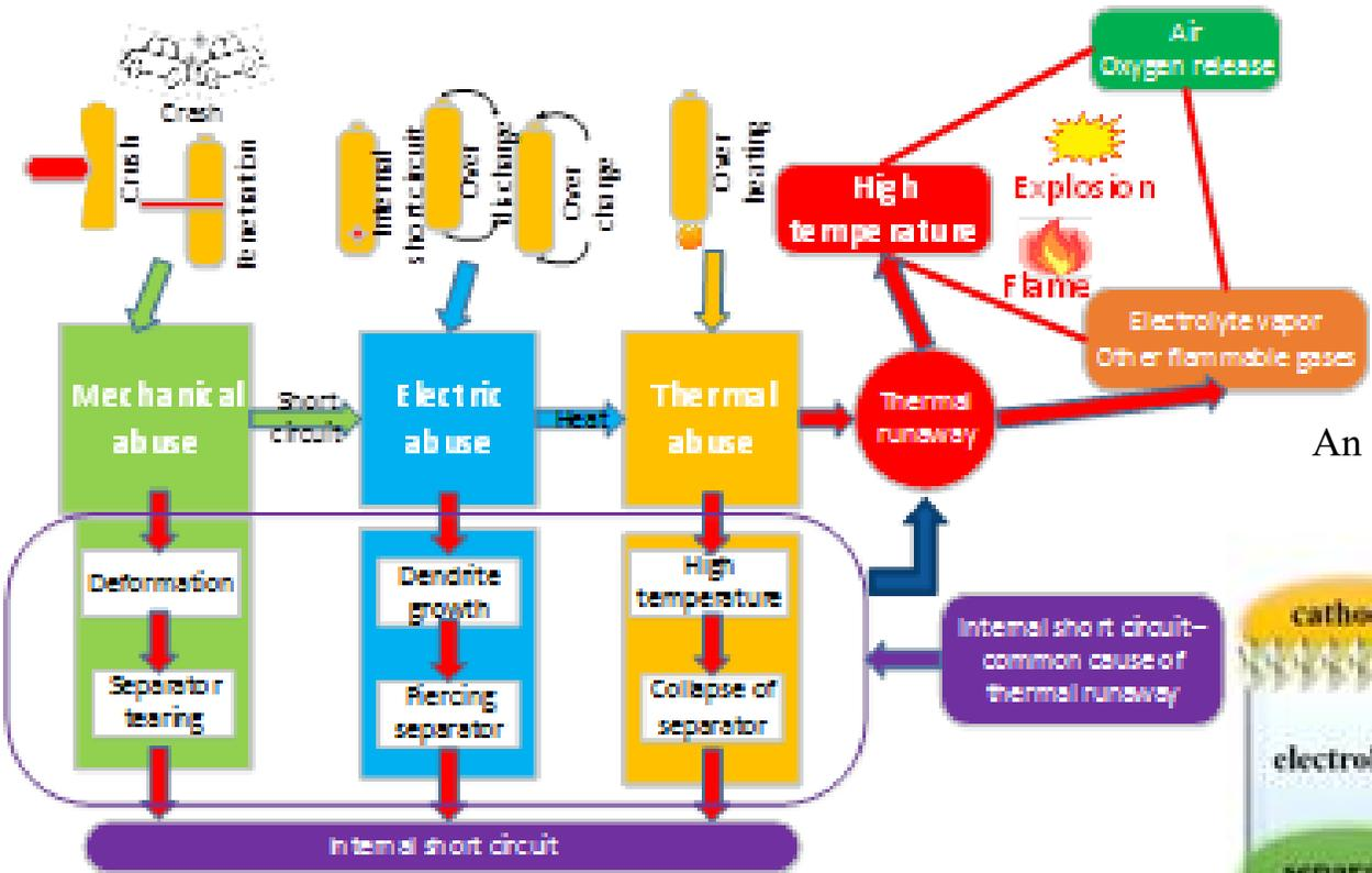
Schematic of the cause of LIB fire accidents
