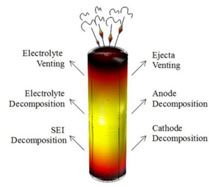
Ref. : Paul T. Coman, Sean Rayman, Ralph E. White, <u>Journal of Power Sources Volume 307</u>, 1 March 2016, Pages 56-62 2 Pressure build up during LiB Cell thermal runaway. 3) Side wall rupture during LiB 18650 cell Thermal runaway
