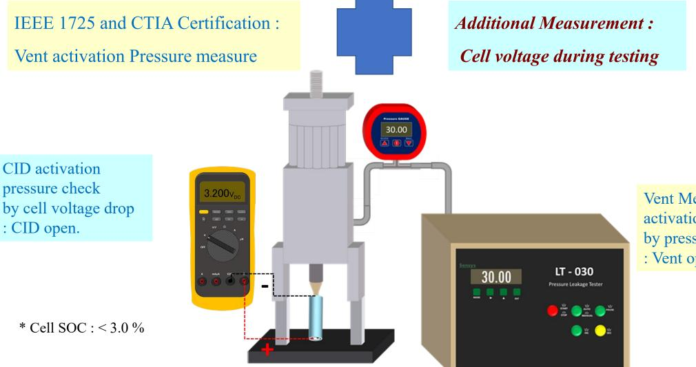
Vent Mechanism activation pressure check by pressure drop : Vent open.
