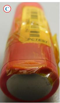
Cell structures were deformed by applied force, but that couldn't lead the cell to the ISC to generate heat and gas. → No CID/Vent activation
