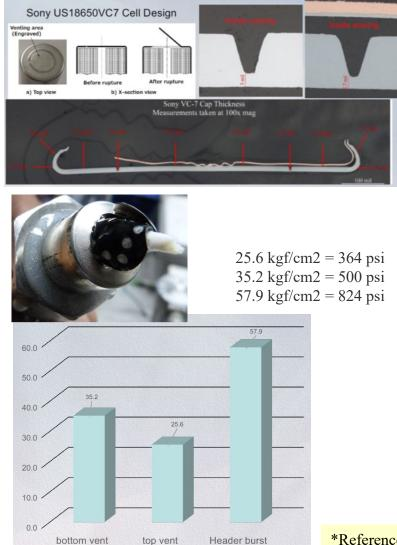
\*Side wall rupture during **Cell Thermal runaway**
