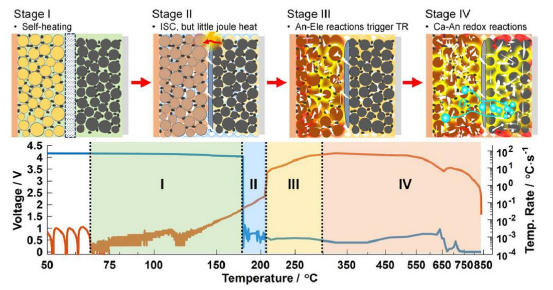
Dongsheng Ren, Xuning Feng, Lishuo Liu, Hungjen Hsu, Languang Lu, Li Wang, Xiangming He, Minggao Ouyang Investigating the relationship between internal short circuit and thermal runaway of lithium-ion batteries under thermal abuse condition, Energy Storage Materials V.34, January 2021, Pages 563-573
