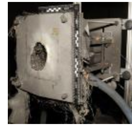
Over Match - Penetration testing 10 mm 2017-T4 Aluminum Sphere @ 6.86 km/s
