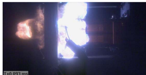
Over Match - Penetration testing 10 mm 2017-T4 Aluminum Sphere @ 6.86 km/s
