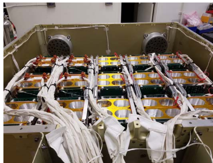
Six live cells, 24 cell simulators
