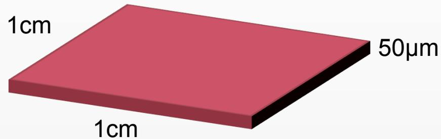
Is the amount of charge held by the active material for a limited cross-sectional area (1 cm x 1 cm) for a specific height (50  $\mu\text{m}$ , which is on the order of Conventional high energy anode thicknesses)<sup>1</sup>.
