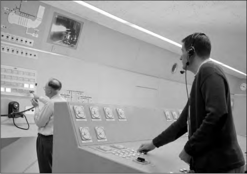
Operations engineers in the control room, located in Building 100, monitor early rocket tests, 1957. Video cameras in the test cell transmitted images during rocket firing. Instruments recorded pressures and other data that was later analyzed by the research engineers in charge of a particular test program. NASA C-45021.
