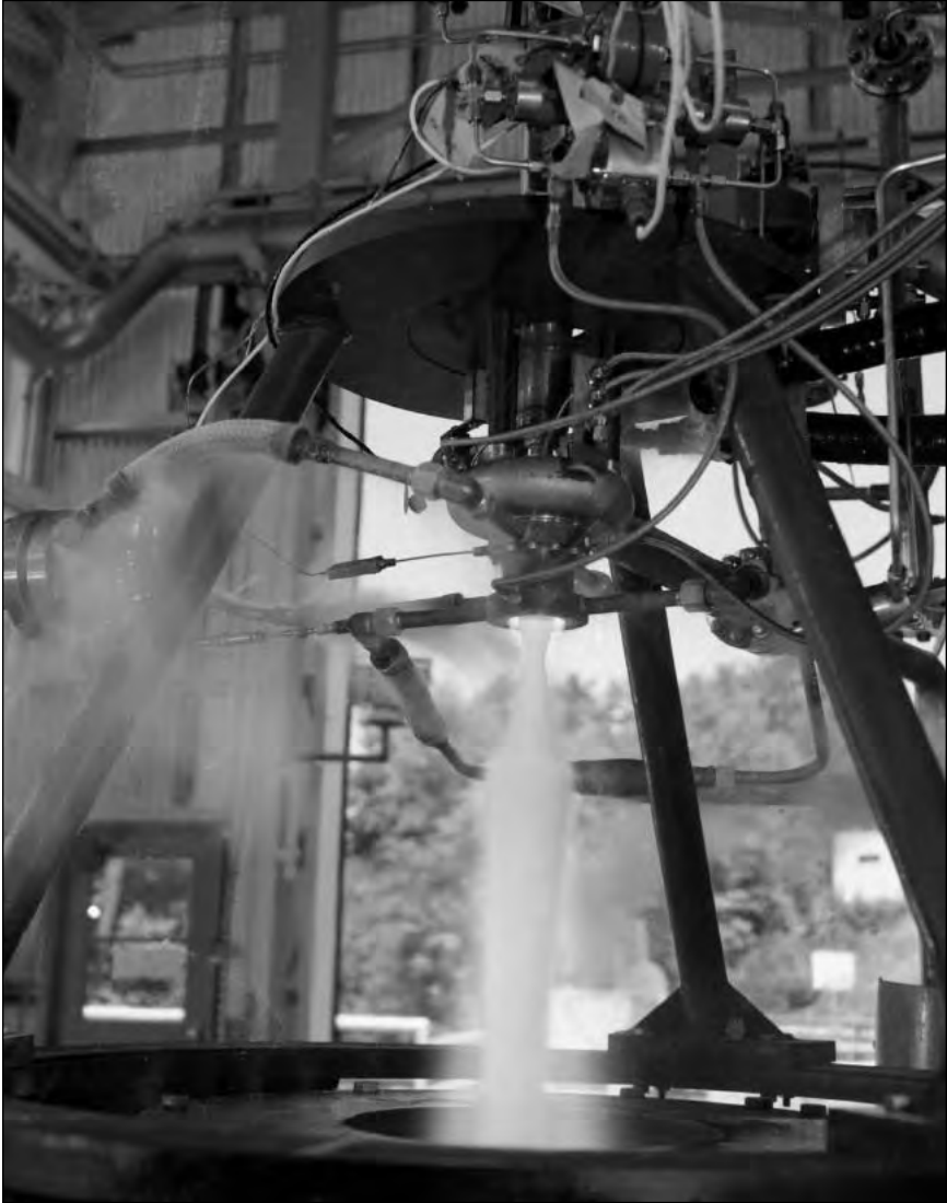
Test of a 5,000-pound-thrust engine used to investigate low cycle thermal fatigue, 4 October 1975. NASA C-75-3125.
