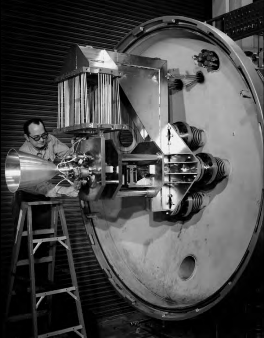
A technician mounts a nozzle on the test stand of the new altitude facility, 1985. The new stand created a space-like vacuum for testing low-thrust engines. It utilized the RETF's existing propellant feed systems, air, water, electrical and data-recording systems. NASA C-85-402.
