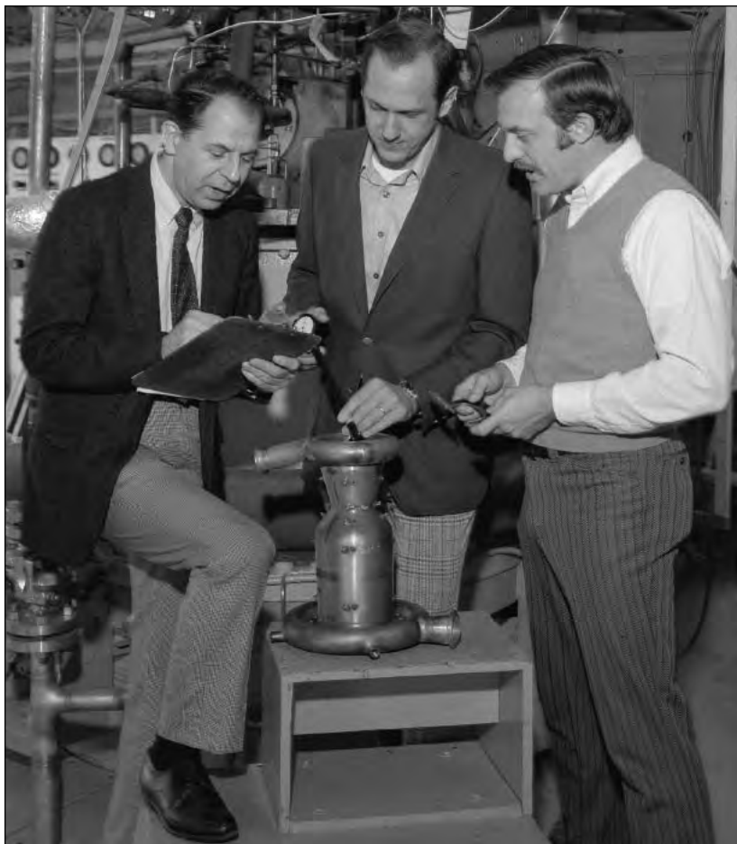
The plug nozzle, used to measure distortion caused by low cycle thermal fatigue, is examined by research engineers Phil Masters (left), Al Pavli (center), and Ned Hannum, 1974. NASA C-74-3466
