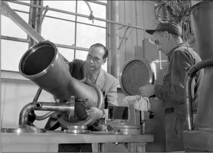
Engineer Walter Russell (left) from the Fabrication Division inspects a regeneratively-cooled thrust chamber for a 20,000-pound-thrust rocket engine while a technician cleans the face plate of an injector in the shop of Building 100, 15 Dec. 1958. NASA C-49343.
