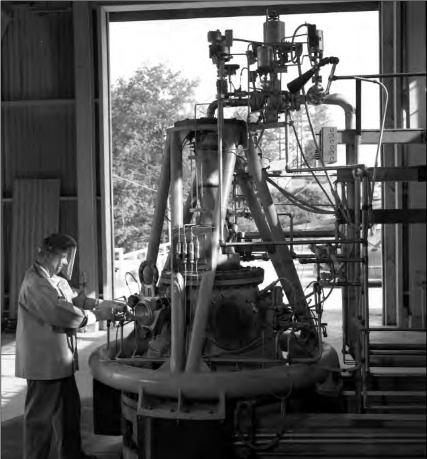
A technician checks the installation of the 20,000-pound-thrust rocket engine on the test stand, October 1957.
