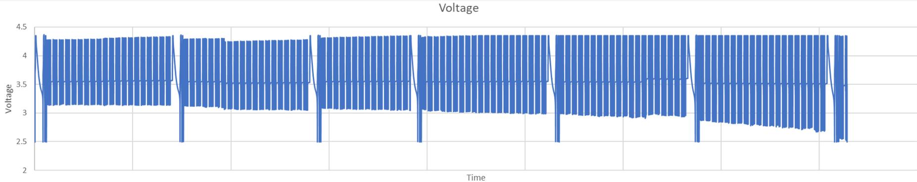
Constant power (eVTOL/Uber protocol): 2E charge, 1E discharge, 4E pulses (E=full energy), ~60% energy cycled; RPT every 200 cycles
