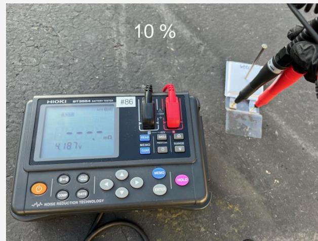
The cells suffer minimal voltage drop during test – nail effectively insulated from electrodes
