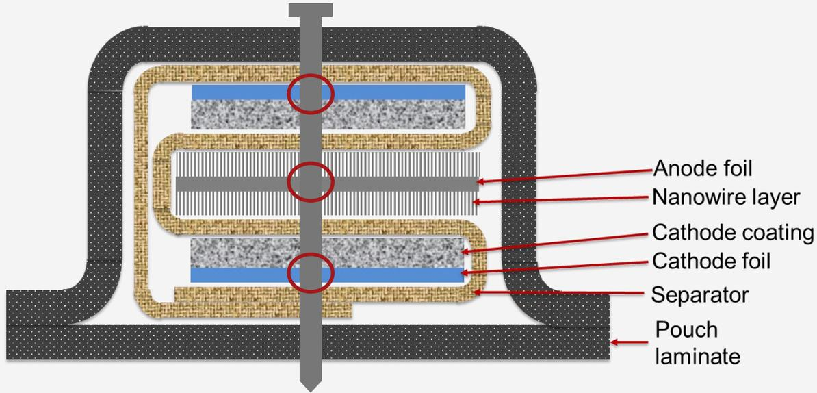
Break/stop short circuit immediately after penetration
