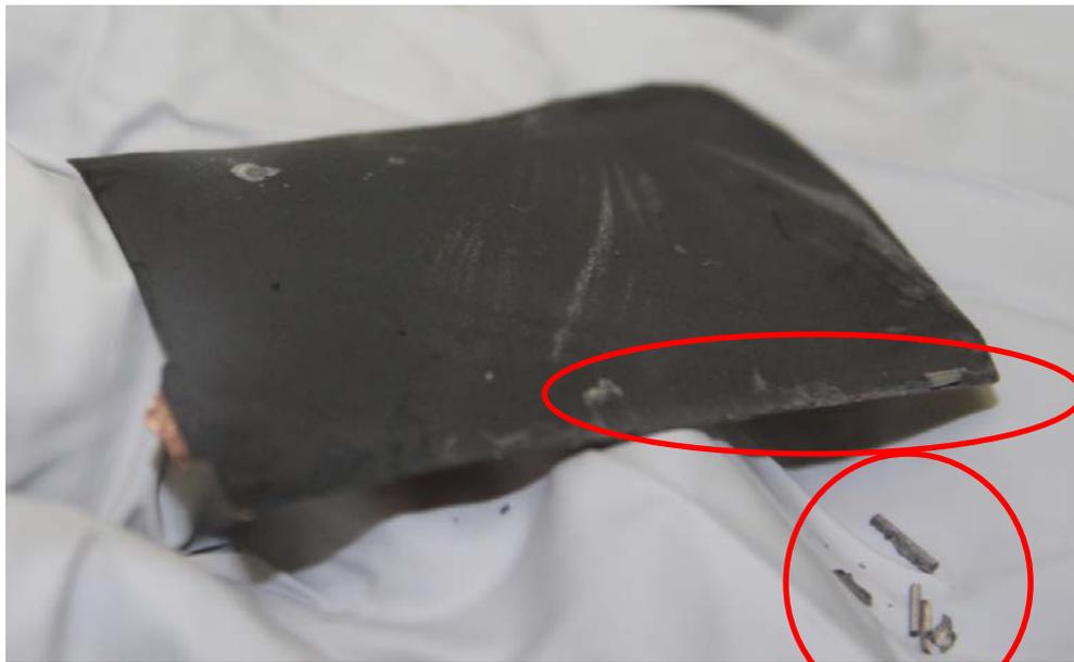
Accumulation of metal like object at the edge of Anode.
