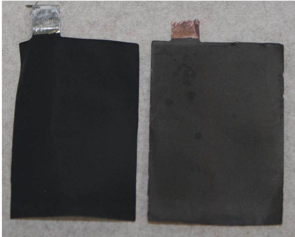
No visible sign of electrode damage or Li plating
