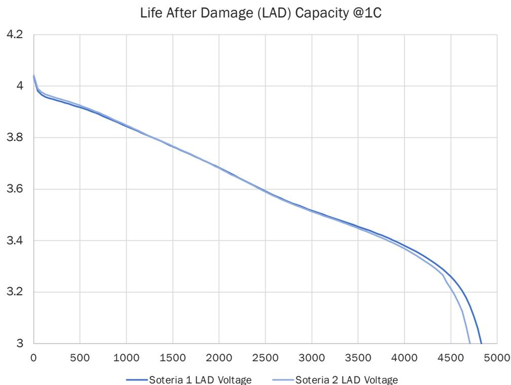
After penetration test, nail was removed & cell was discharged at C rate.
