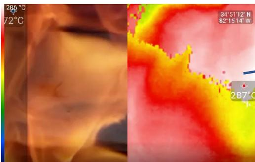
Control cells exhibited typical thermal runaway behavior
