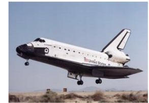
Figure 23: On reentry from space, the space shuttle orbiter did not use engines and landed as a glider.
