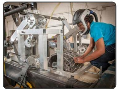
These test rigs are used to study how rover wheels operate in simulated extraterrestrial soils. For example, engineers are studying how damage on the wheels of the Curiosity rover affects its mobility as it explores Mars.
