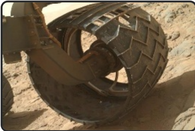
This photograph, taken from the underside of the Curiosity rover sitting on Mars, clearly shows puncture damage on the treads of the aluminum wheel.
