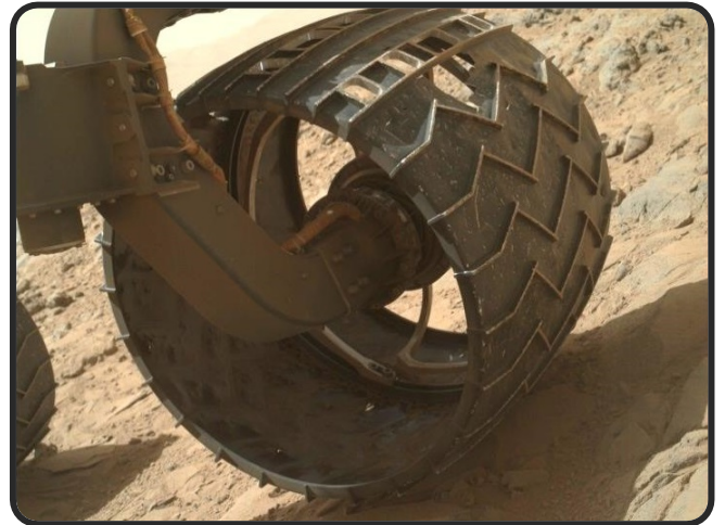
Close-up of one of the Curiosity rover’s wheels on Mars. Some damage is noticeable near the top of the image.
