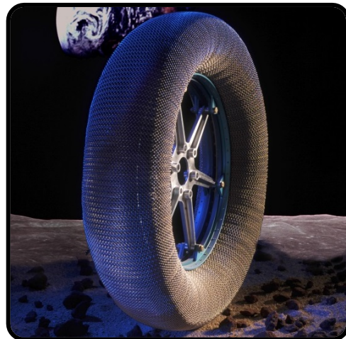
Airless tire developed and tested by NASA and Goodyear
