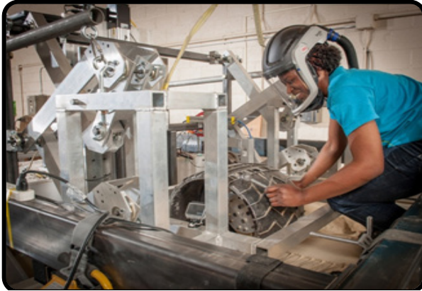
GRC technician conducting a test on a simulated Curiosity rover wheel in the TREC rig.
