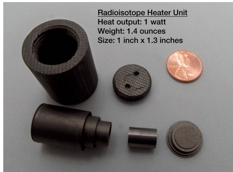
Figure 2-7. Radioisotope Heater Unit
