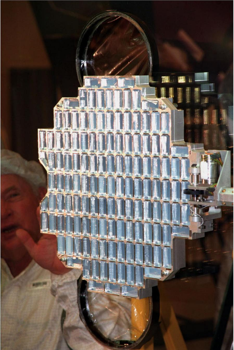
**Figure 2-3: Aerogel in the Payload Hazardous Servicing Facility**
