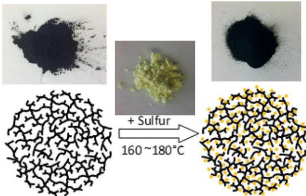
**Porous, conductive** ceramic host with **high affinity** to sulfur and polysulfides
