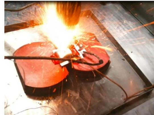
2Ah Li S cell (left )and 2Ah Li ion cell (right) nail penetration tests
