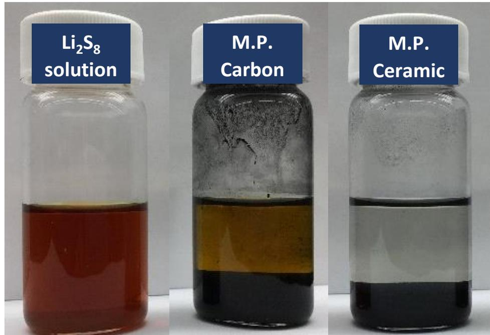
Sealed vials of Li<sub>2</sub>S<sub>8</sub> solution, and after contact with ceramic and mesoporous carbon overnight
