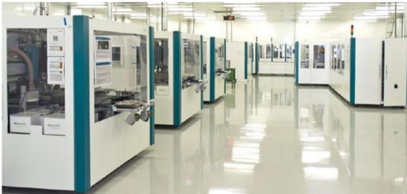
Navitas' \$15M state of the art automated production facility with the capability of producing up to 1M+ custom format pouch cells per year with 1 – 10 Ah capacity
