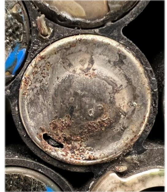
**Run 1, Trigger Cell #112:** Cell experienced SWR, SGR and BR. Minor damage to bore anodization but no perforations in aluminum.
