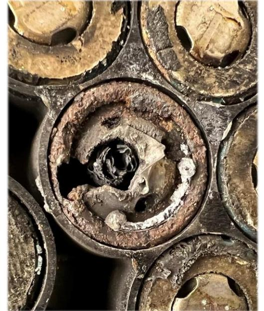
**Run 4, Trigger Cell #91:** Large SWR and SGR observed on cell along with hole in aluminum bore. Lends explanation for shorted adjacent cell (0V cell).
