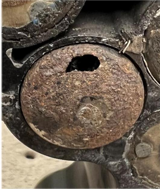
**Run 6, Trigger Cell #20:** Header assembly release, no SWR or SGR but had BR. No bore damage.
