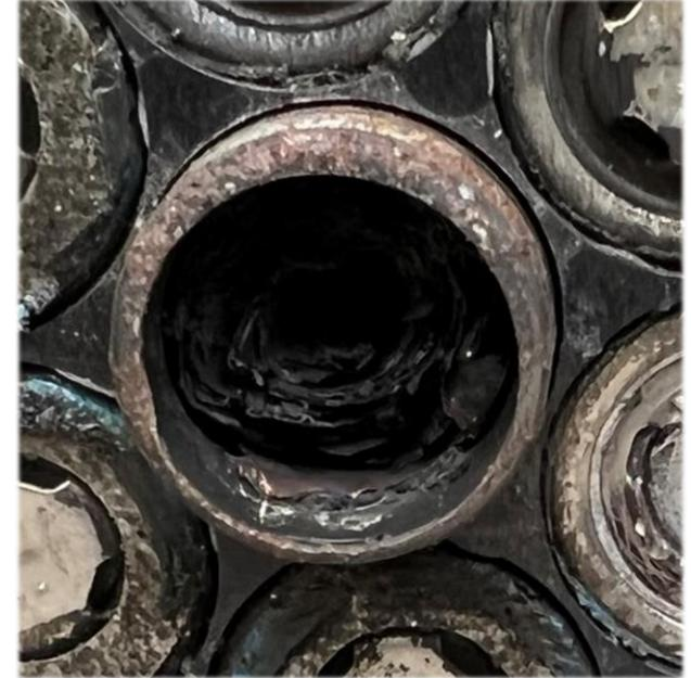
**Run 10, Trigger Cell #6:** Cell experienced SWR and BR but no SGR. No damage observed to bore. Header release occurred during TR.
