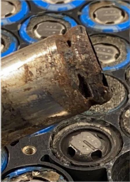
**Run 2, Trigger Cell #16:** Multiple SGRs, no visible damage to bore.
