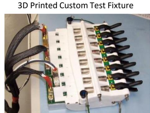
3D Printed Custom Test Fixture
