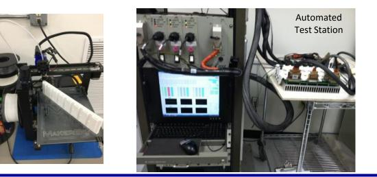
3D Printed Custom Test Fixture
