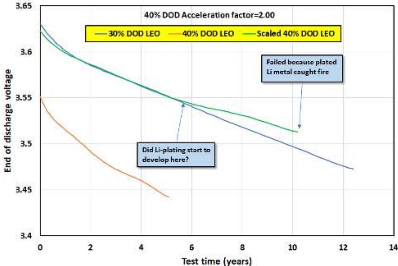
*Increase in discharge voltage trajectory for 40% DOD could have given ~2 year warning prior to cell failure, if compared to 30% DOD trajectory*
