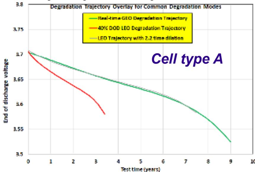
*Failure verified by DPA to result from capacity loss due to SEI growth in both 40% DOD LEO and real-time GEO life tests*
