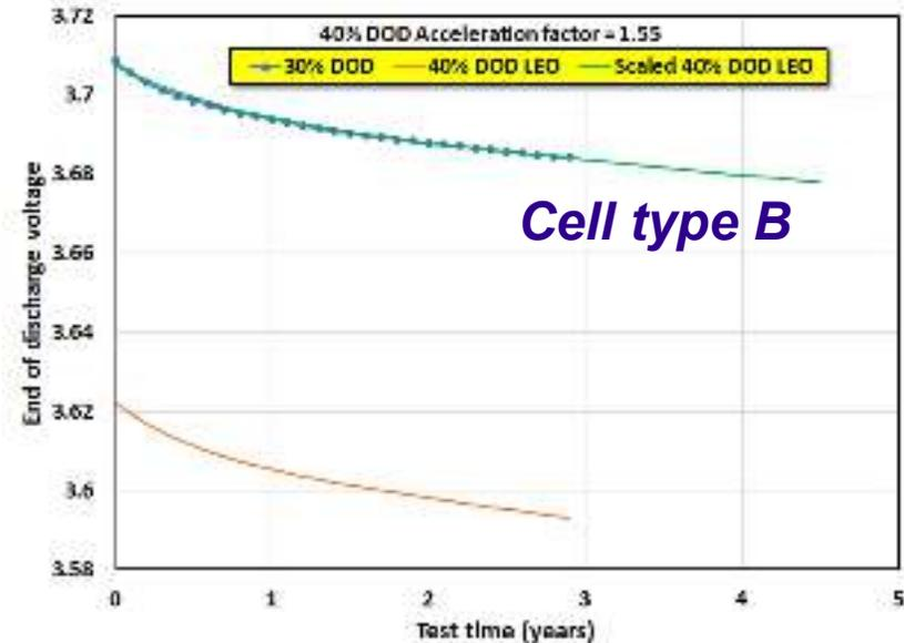
*Failure is expected to be caused by the same processes at both 30% and 40% DOD, because trajectories overlay each other*
