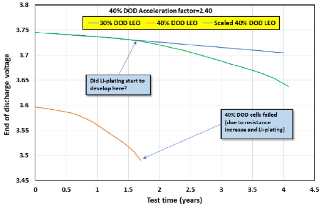
*Li-Ion cell shown here failed quickly in 40% DOD LEO profile due to resistance increase and Li-plating, but ran without failure at 30% DOD*
