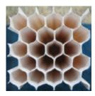
the tall grass reeds common in wetlands. Experiments have shown that bundles of reeds are good at absorbing sounds, but there is one big problem. Natural grass reeds are not durable enough to withstand the super-hot, high-pressure environment inside a jet engine. Danielle and her team are working to get the same effects as grass reeds, but with materials that can withstand the heat of an engine.
