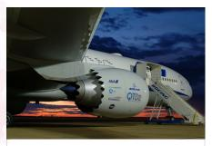
Another way NASA has reduced jet engine noise, which Danielle helped research, is seen on this Boeing 787. The saw-toothed cuts at the back of the engine change how the jet's hot exhaust mixes with cold outside air. That makes the engine quieter.
