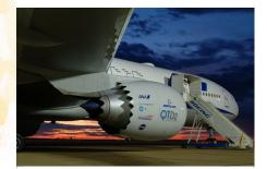
Another way NASA has reduced jet engine noise, which Danielle helped research, is seen on this Boeing 787. The saw-toothed cuts at the back of the engine change how the jet's hot exhaust mixes with cold outside air. That makes the engine quieter.
