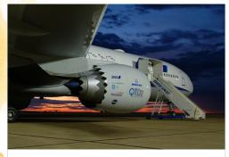
Another way NASA has reduced jet engine noise, which Danielle helped research, is seen on this Boeing 787. The saw-toothed cuts at the back of the engine change how the jet's hot exhaust mixes with cold outside air. That makes the engine quieter.
